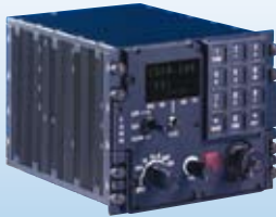
F 3 – ARC 164 10 W – local control
